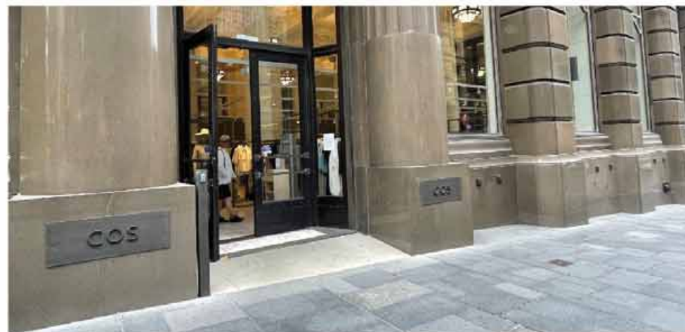
Fig. 6.2251 The sloping terrain in front of 17 Martin Place was overcome by raising the available footpath to floor level without providing excessive gradients.
